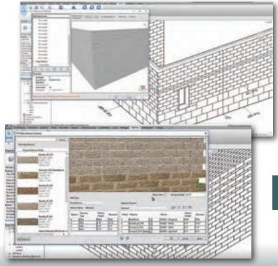
Custom Bond Patterns Analyze Layout Geometry True Masonry Sections Render Masonry Materials
